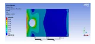
According to the contour plot, the maximum stress at fastener hole due to applied the loads. The maximum stress is 356.35N/mm<sup>2</sup> and minimum is 0.085787N/mm<sup>2</sup>
